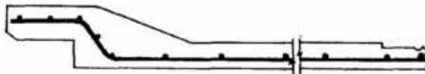
3C Cage made of Continuous Longitudinals
