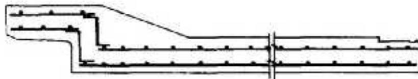
FIG. 3 TYPICAL ARRANGEMENTS OF REINFORCEMENT IN SOCKET FOR SINGLE CAGE
