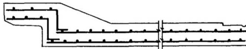
4B Socket Cage Longitudinal Suitably Bent for Connecting to Barrel Cage
